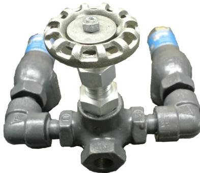
**DUAL ASSEMBLY WITH UNIONS (DU):** Includes two (2) relief valves, one (1) three-way manifold shut-off valve, four (4) 90° elbows, four (4) unions, one “tee” and twelve (12) nipples. (Assemblies using relief valves with male NPT inlets have only ten (10) nipples.) Only one side of the three-way valve can be closed at any time. This assembly will allow either valve to be changed without disturbing the piping.
